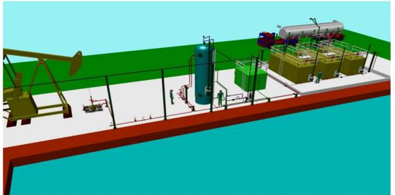
Figure 1: Production site layout incorporating (from left) pumpjack, heater treater, water knockout tank, crude storage tanks and offloading to road tanker
