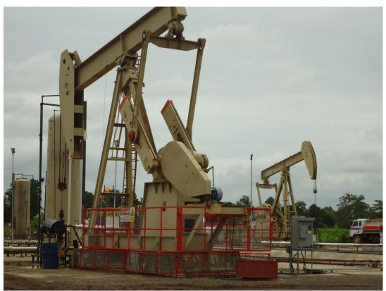
Figure 5: Multiple production wells per location
